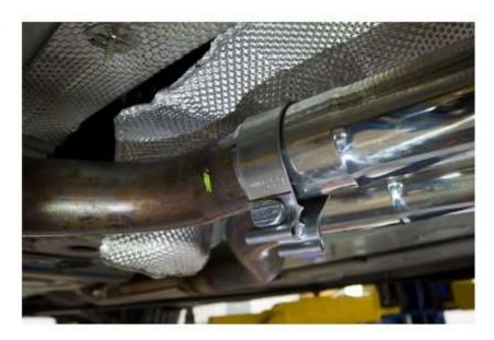
8. Align and slip URUTU X-Pipe onto rear factory tubing.
