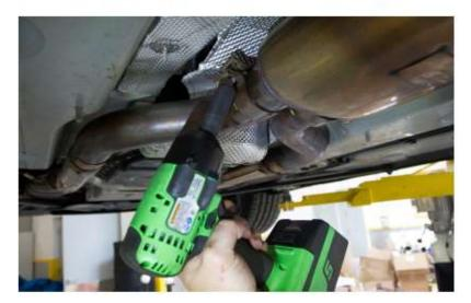
5. Separate exhaust sections at the rear joint. (NOTE: A rubber mallet may be needed to tap the sections apart)
