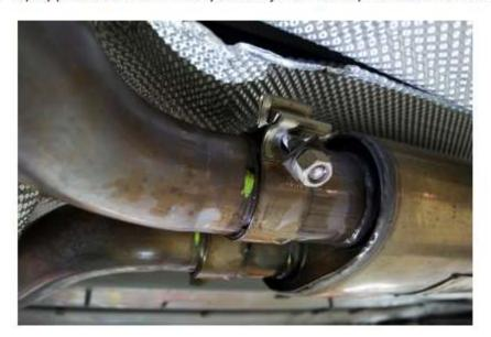
3. Loosen rear exhaust joint clamps aft of the factory resonator.
