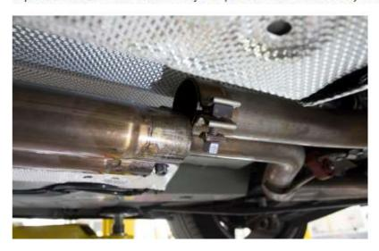
6. Separate the front joint of the resonator section and remove the factory resonator.
