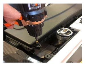
3) Position the URUTU lid on the air box and ensure the edge of both air filters goes into the curved cavity of the lid, then make sure all the screw holes on the lid and the bottom section of the air box are fully aligned
