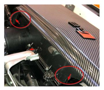
4) Start driving the screws into place, but do not fully torque until you have ensured the lid is properly seated and making full contact with the bottom section of the air box (if using a power drill be careful not to let the rotating part of the drill make contact with the lid or damaged can be caused). Lastly, be careful not over torque the screws otherwise you might strip the tread on the bottom section of the airbox.
