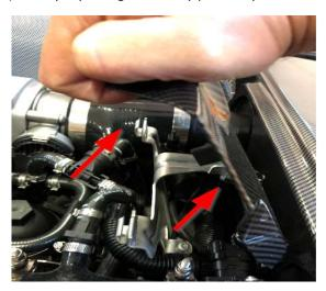
2) Using the Hex-bit driver and/or electric drill and T25 hex-bit remove the 10 screws that secure the lid to the air box and remove it by lifting it upwards and away from the airbox assembly.
