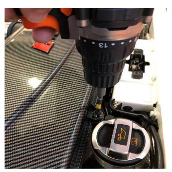
5) Secure the vanity plate in place by aligning the rear tab (the single one closest to the air box) with the receiving metal bracket, then align the two other tabs
