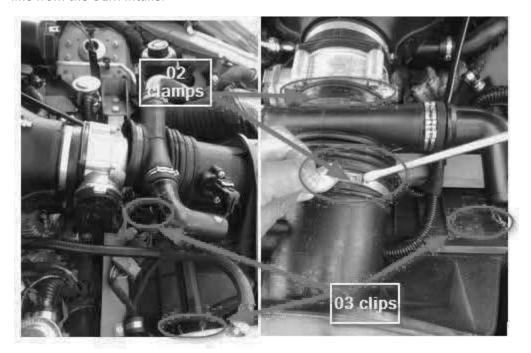
3. Remove the OEM intake and install the URUTU replacement unit (you may use a screwdriver to facilitate the process)
