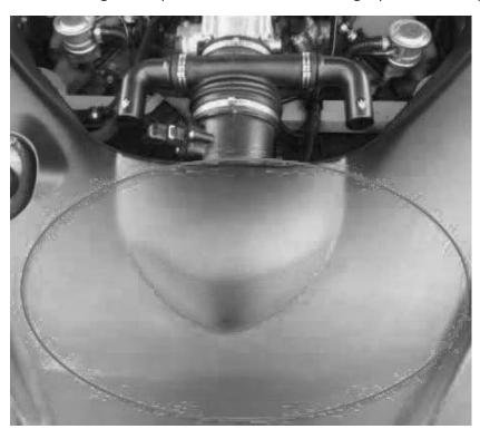
2. Loosen up the three clips-latch that secure the air box in place and remove the two hose clamps and the vacuum line from the OEM intake.
