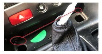
14) Only one more screw remains holding the dash in place, to access it you need to remove the plastic cover under the steering column, remove the three screws at the bottom, then use a plastic pry tool to gently separate the bottom from the top section, once the bottom comes off the last scree will be exposed on the side of the dash on the right side near the ignition
