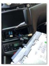
7) Remove two additional screws that sit diagonally behind the radio
