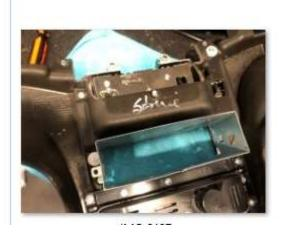
16) Remove the screen assembly / bezel and move all components onto the URUTU bezel being careful NOT to over torque or you will strip the brass treaded mounting points (this is true for both OEM or aftermarket bezels)
