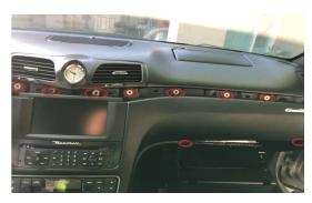
4) Now that the clock trim is exposed and the bottom screws removed use a pry tool to pull the clock assembly out and disconnect the clock wire (the upper section is held in place by pressure clips) -
