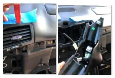
5) Remove the 3 metal clips, the AC vents and the clock from the OEM assembly and transfer over to the URUTU clock bezel using the factory screws
