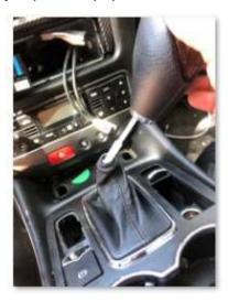
12) Using a plastic pry tool carefully remove the side panels on either side of the center console, they are held in place by pressure clips (refer to tips and trick section of this tutorial about panels sticking together, do not yank abruptly or you can damage the leather)
