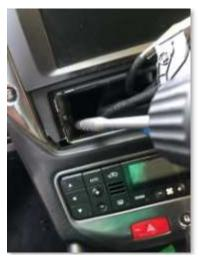
8) Using a plastic pry tool remove the rubber cover at the bottom of the AC controls and then remove the screws exposed behind it
