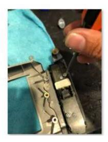
17) Mount the screen assembly with the URUTU bezel onto the large dash section
