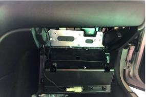
2) Using a plastic pry tool remove the larger trim piece that sits horizontally across the dash, this is a metal piece coated with different finishes, it will not break or bend (it is held in place with pressure clips)
