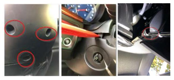
15) Pull the entire dash slightly forward towards you and disconnect the wires from the back of the screen and AC controls, then take the entire assembly out of the vehicle
