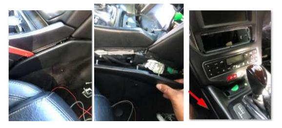
13) Pull the center tray back and if needed disconnect the gear indicator wire (do not disconnect the e-brake wire or it will be de-programmed), pulling the center tray back will expose 2 more screes holding the dash to the frame
