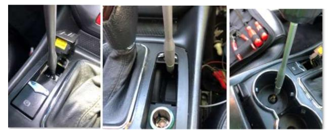
11) Remove the shift knob by pulling upwards (it is not screwed in place, do not twist on or you will break something, just pull firmly upwards and it will come off)
