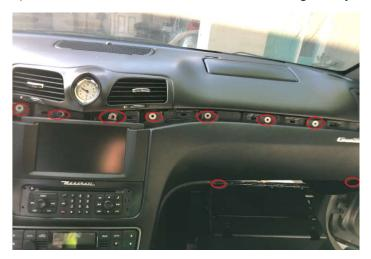
3) Now that the clock trim is exposed, and the bottom screws removed use a pry tool to pull the clock assembly out and disconnect the clock wire (the upper section is held in place by pressure clips)
