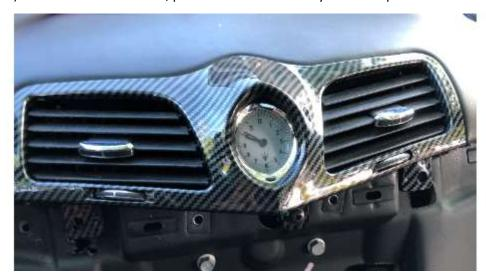
6) Put all screws back in the original place, and press the larger trim back into place
