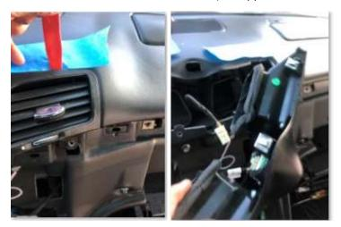
4) Remove the 3 metal clips, the air vents and the clock from the OEM assembly and transfer over to the URUTU clock bezel
