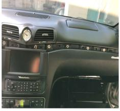
2) Remove the screws that were behind the large trim just removed
