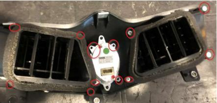
5) Connect the clock wire, press the entire assembly back into place and ensure the fit is flush
