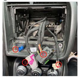
4.Use the removal tool to pry off the frame
