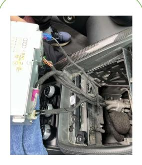
3. Disconnect the plug to connect the host. Unplug the OEM head unit
