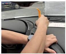
6. Remove screws to remove AC vents
